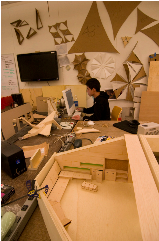
Figure 5. The F-Stop Studio worked across numerous scales from full-scale sketch models in the background, prototype assemblies in the middle ground, to highly precise model-as-prototype in the foreground laser-cut from full-scale fabrication cut files as a test of construction prior to full-scale fabrication and assembly.
